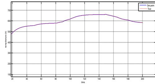
Figure9. Controlled output  $T_{out}$  and set point for June
