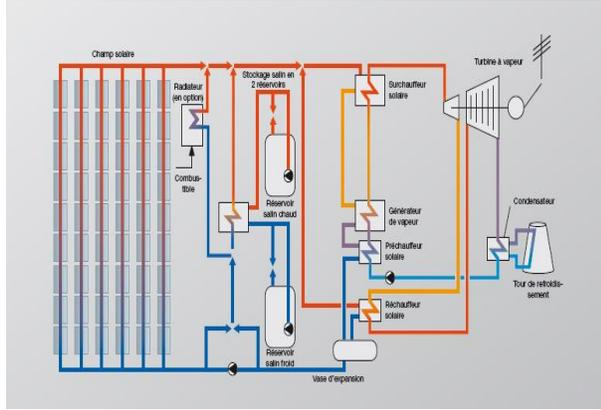
**Figure 1.** Flow Diagram of the 30 MWe SEGS VI Plant for Pure Solar Model.
