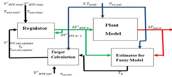
Figure6. T-S fuzzy MPC Controller
