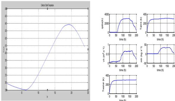
Figure 4, The input system and the collector outlet temperature of the Solar collector Field
