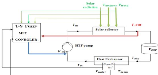
Figure5. Block Diagram with Plant Model and Controller.
