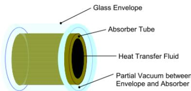
**Figure 2.** The Heat Collection Element.
