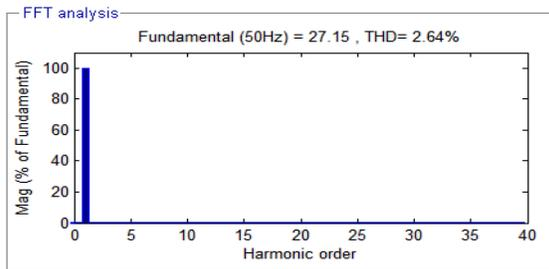
Fig.6 Spectrum harmonic of line current
