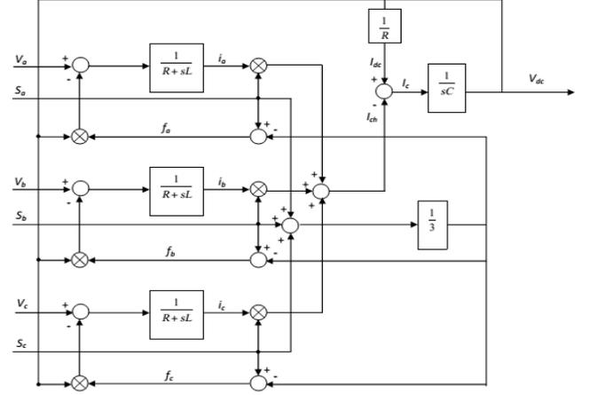
Fig. 2 Block diagram of voltage source PWM rectifier
