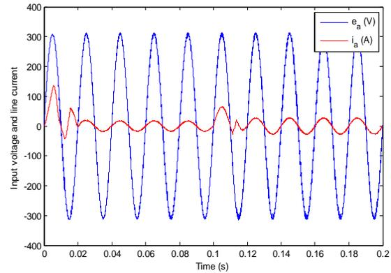
Fig.7 Input voltage and line current superposition
