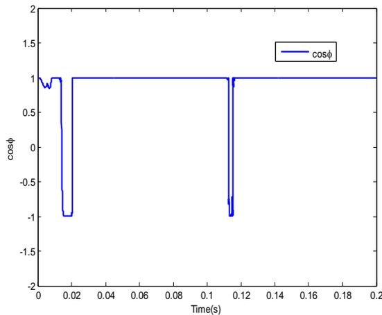
Fig.10 Power factor of PWM rectifier
