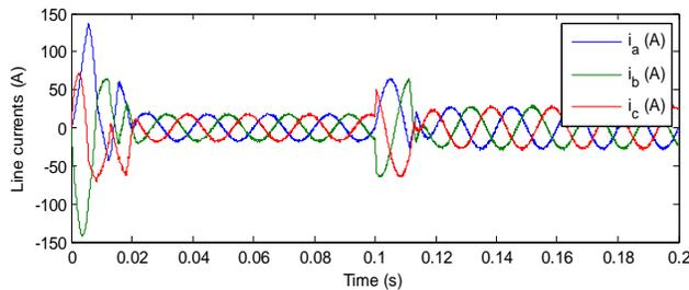
Fig.5 Line input current of PWM rectifier
