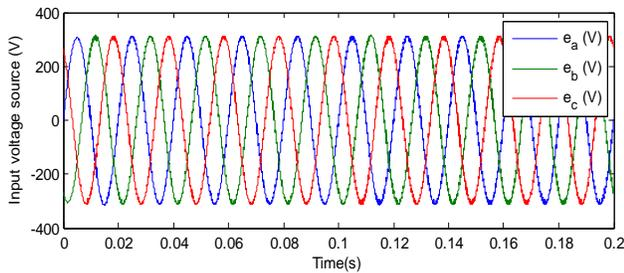
Fig.4 The input voltage of PWM rectifier
